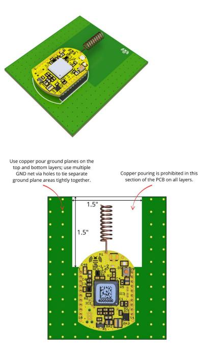
Sockets can be used on the host circuit board for ease of removing and replacing WillowBee. Alternatively, WillowBee can be soldered directly to the host circuit board.
