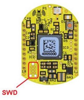
**Push Button:** Push button is connected to port PA0 of the microcontroller which also acts as ON/OFF pin to wake up the microcontroller. One of the alternate functions of PA0 pin is wakeup function (WKUP1).
