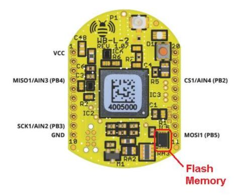
**UART:** Dual hardware UART's. UART1 on pins 2 and 3. UART2 on pins 7 and 8. Combined with BOOT (pin 6) and NRST (pin 5), UART2 allows firmware download to WillowBee over UART2.
